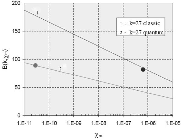
Figure 4: Diffusion factor  $B$  as a function of the  $\chi_m$  parameter in the classic and quantum approximations. The bold points on curves correspond to the CLIC parameters: 2.242 GeV beam energy, 0.34 mA beam current per bunch and 0.003 ratio of the vertical and radial emittances.
