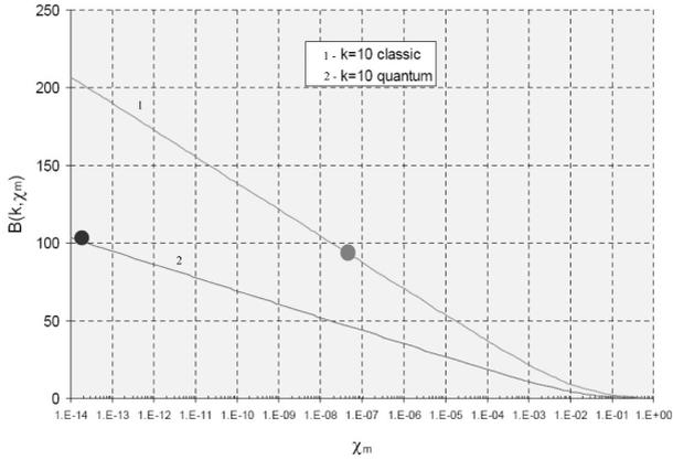
Figure 5: Diffusion factor for the VEPP-4M vs the  $\chi_m$  parameter in the classic and quantum approximations at 0.9 GeV, 0.1 mA per bunch and 0.01 ratio of the emittances (the bold points on curves).
