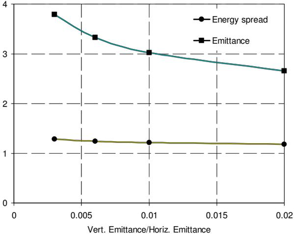
Figure 3: Relative increase of the beam emittance and energy spread due to IBS versus the ratio of vertical and horizontal beam emittances for the CLIC Damping Ring at  $E = 2.24$  GeV and  $I = 0.34$  mA/bunch
