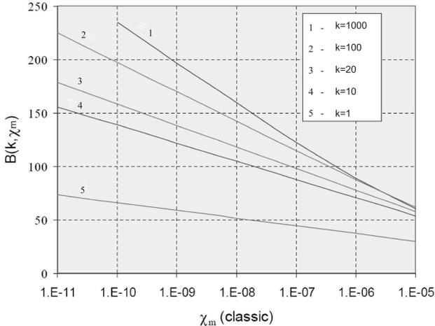
Figure 2: Diffusion factor vs  $\chi_m$  in the approximation of classic lower limit on the scattering angle at some values of the coupling parameter  $k$ .
