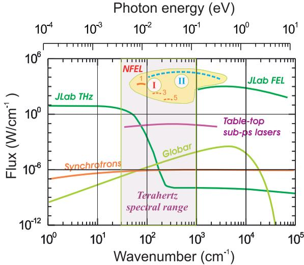
Figure 1: Spectral power density of the terahertz sources. The curve 1 corresponds to the first harmonic of NFEL radiation. The curves labelled with figures 3 and 5 show expected flux of third and fifth harmonics. The dashed curve is the project flux of the NFEL second stage.
