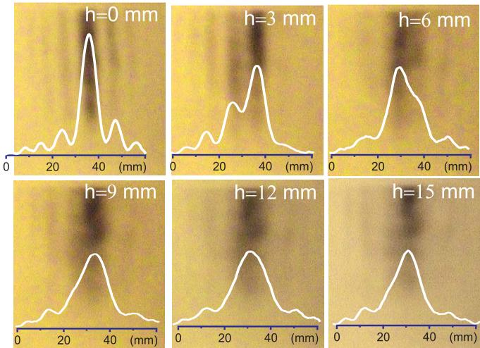
Figure 5: Interference patterns formed by terahertz laser radiation reflected from a Fresnel bi-mirror ( $h$  is the longitudinal displacement of one of the mirrors). The images are recorded with a digital video camera SONY DCR-TRV230E using a Thermal Image Plate (detector of radiation based on thermal quenching of phosphor luminescence).
