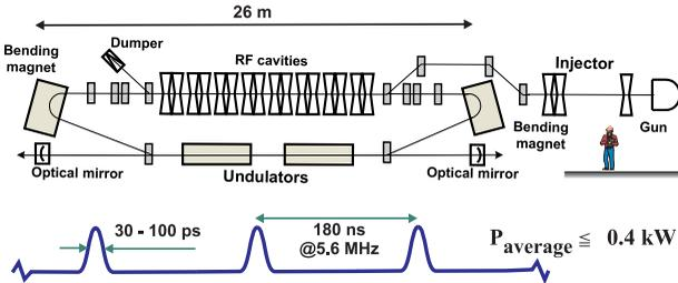
Figure 2: Schematic of the Novosibirsk terahertz free electron laser and radiation intensity vs. time.
