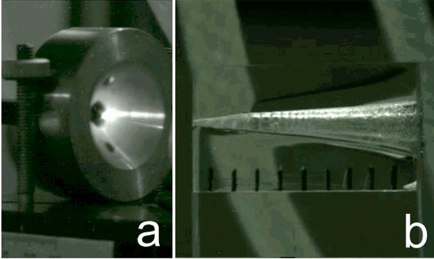
Figure 3: Interaction of the laser radiation with matter: (a) continuous optical discharge in the focus of a parabolic mirror and (b) the opening in PMMA drilled by non-focused laser beam; distance between the marks is 5 mm. In this experiments the wavelength was  $130 \mu\text{m}$  and the average power of radiation was about 100 W.
