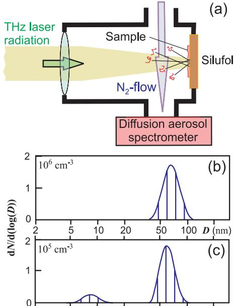
Figure 4: Ultra-soft laser ablation of DNA samples on silufol. (a) The experimental configuration. Size distribution of ablative material recorded with a diffusion aerosol spectrometer for two samples containing (b) a phage DNA and (c) a mixture of the phage DNA with a plasmide DNA (size ratio is close to ten). Wavelength –  $120 \mu\text{m}$ , power density -  $20 \text{ W}/\text{cm}^2$ .
