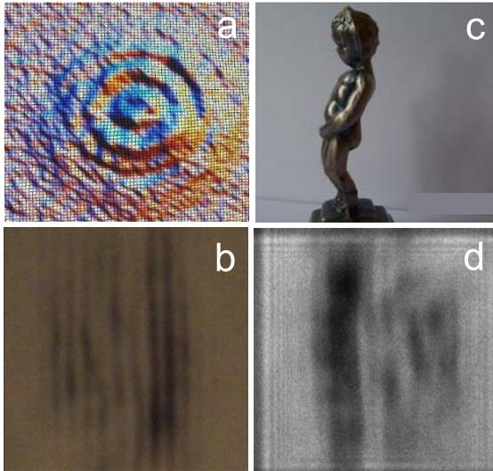
Figure 6: Application of the TIP imager (surf. No. 6) to terahertz holography: (a) 3D-plot of the terahertz beam reflected from a spherical mirror with a 4.5-mm opening at the center; (b) a hologram recorded when a small statuette (c) was posted in front of one of the Fresnel mirrors; (d) the image digitally retrieved from the hologram.
