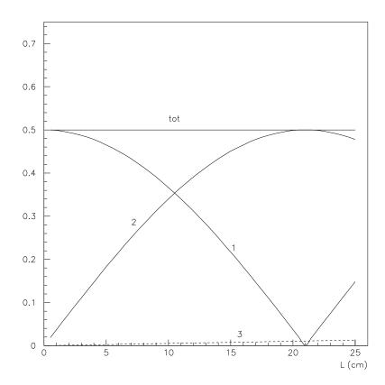
Figure 4: Absolute values of the Stokes parameters  $\mid \eta_1(L) \mid$  (curve 1),  $\mid \eta_2(L) \mid$  (curve 2),  $\mid \eta_3(L) \mid$  (curve 3), and the polarization degree  $\mid \boldsymbol{\eta}(L) \mid$  (curve "tot" ) depending on the thickness L of a silicon crystal at  $\omega = 100$  GeV,  $\eta_1 = -0.5$ ,  $\eta_2 = \eta_3 = 0$ ,  $\vartheta_0 = 2.29$  mrad,  $\varphi_0 = 0$ .
