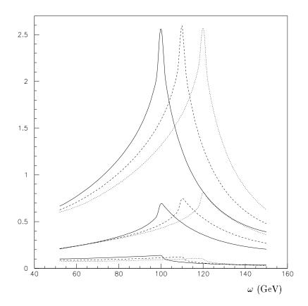
Figure 3: FOM (upper curves), FRAC (lower curves), and the degree of circular polarization  $\xi$  for  $\varphi_0 = 0$  near < 110 > axis of a 10 cm thick silicon crystal as functions of  $\omega$  (GeV). Three sets of curves (from the left to the right) correspond to the angles of incidence  $\vartheta_0$  (mrad) = 2.29, 2.08 and 1.91 respectively.
