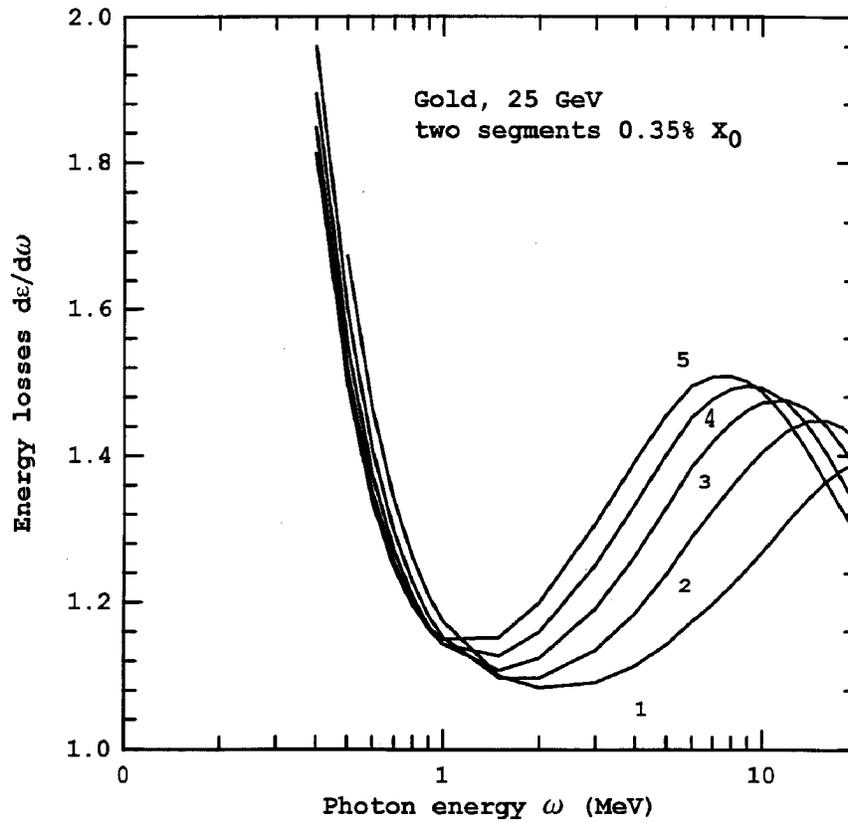
Figure 1: The energy losses spectrum  $\frac{d\varepsilon}{d\omega}$  in units  $\frac{2\alpha}{\pi}$ , in the target consisting of two gold plates with thickness  $l_1 = 11.5 \mu\text{m}$  for the initial electrons energy  $\varepsilon=25 \text{ GeV}$ :
