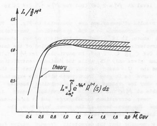
Fig. 2. Comparison of the first sum rule with the experiment.
