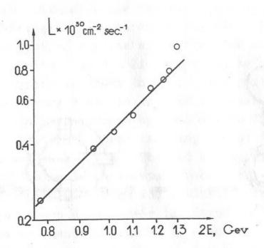
Fig.2 Energy dependence of luminosity.
