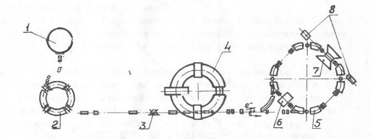
Fig.1 Lay-out of VEPP-2M complex: 1 - injector ILU;
