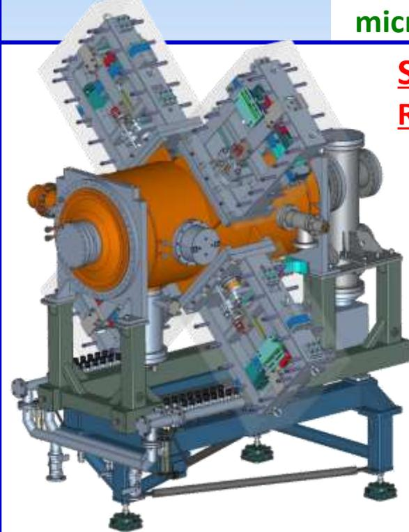
**Step 2:** Formation of the short ion bunches at presence of cooling: RF-2 (100 kV, 4 cavities) from *coasting beam* to  $\Rightarrow$  **22<sup>nd</sup> harmonics**
