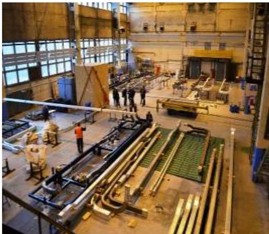
Aluminum busbars PF / CS, SS at the assembly site for Bld.32,33
