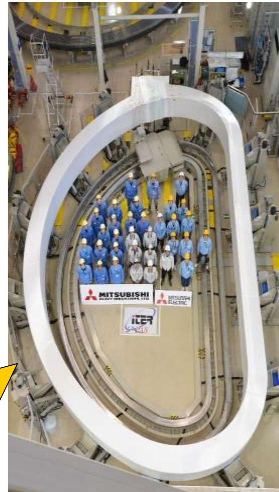
Insulation wrapping of 7 DPs stacked for first JA TF Coil was completed in January 2017, which is timely accomplishment of one of the IC milestones.
