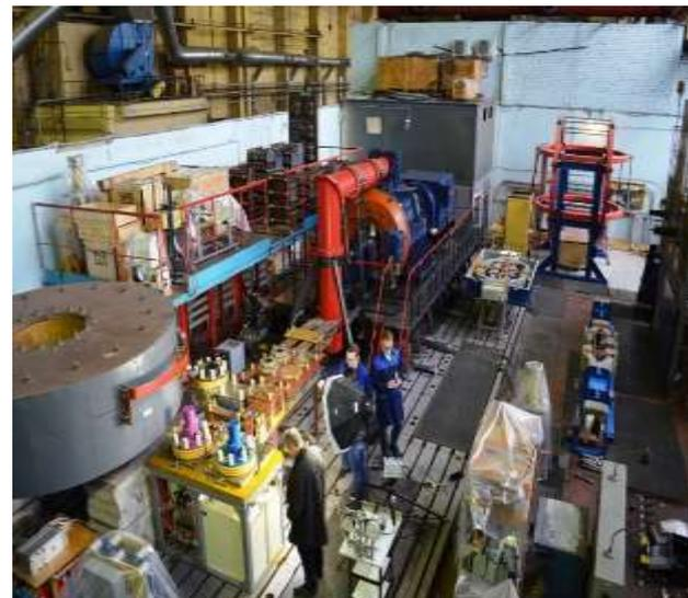
Test facility for circuit breaker
