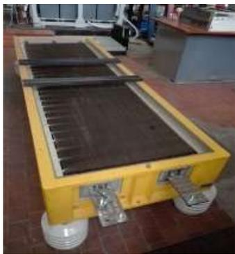
Section of the SNR CS1 resistor assembly
