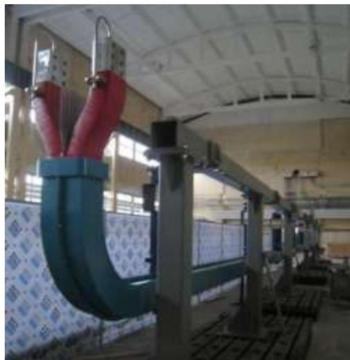
Busbars—the components that connect the superconducting magnets with their power supply—are capable of carrying 70kA of current.
