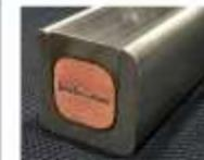
Helium gas cooled HTS conductor
