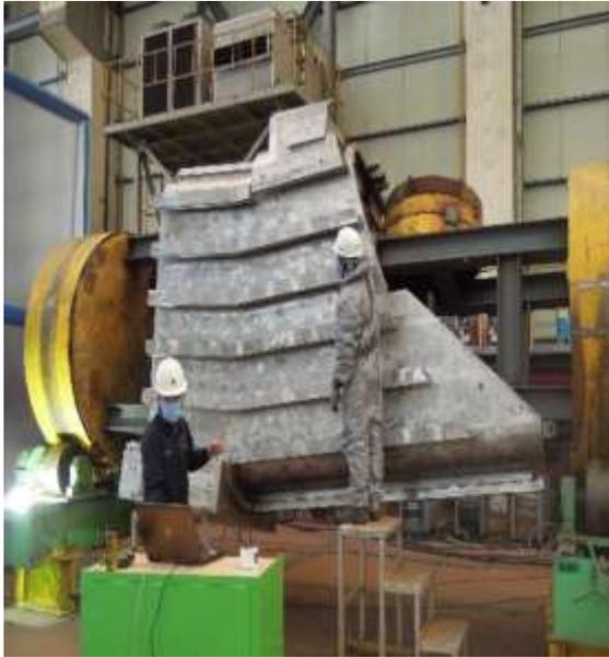
T-rib to Inner Shell assembly of LPSE
