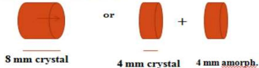
Both kinds of targets have been tested at CERN. The positron yield was the same for the 8 mm crystal as for the (4 crystal + 4 amorphous) .
