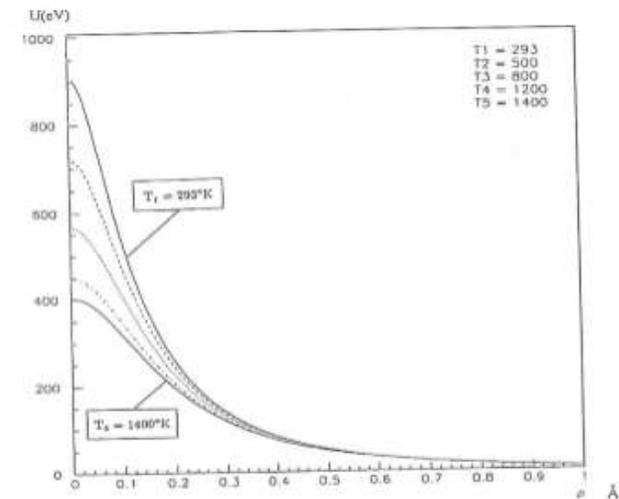
FIGURE 9 Continuum potentials for the  $\langle 111 \rangle$  axis of the tungsten crystal. The temperatures are expressed in K.
