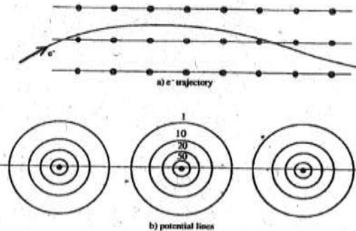
Figure 10 : Axial channeling on a Si  $\langle 111 \rangle$  crystal.
