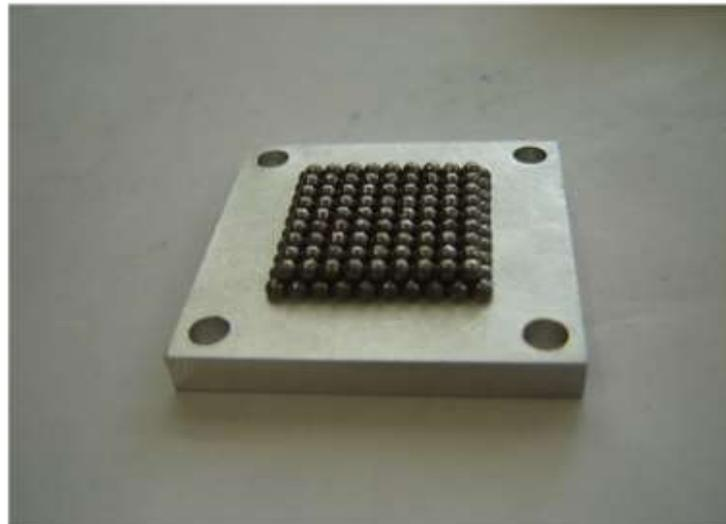
With respect to bulk targets a granular target made of small spheres ( $\phi \sim 1$  mm) presents better heat dissipation
