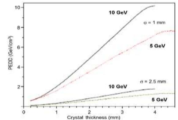
Fig. 4. PEDD versus crystal thickness for  $E = 5$  and 10 GeV. For the upper curves, the r.m.s. incident beam radius is 1 mm and for the bottom curves, 2.5 mm.
