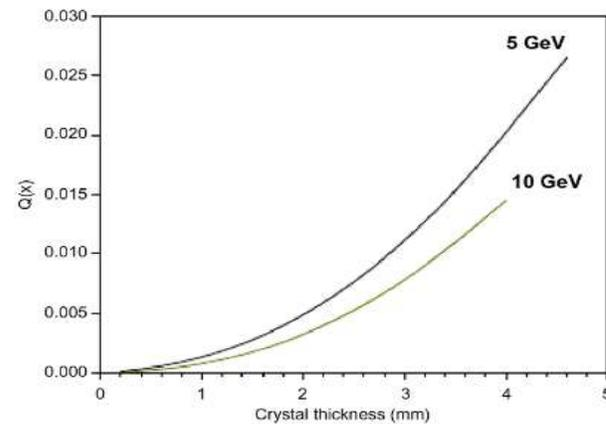
Fig. 3. Total energy deposited in the radiator: ratio  $Q(x) - E_{\text{dep}}/E$  for  $E = 5$  and 10 GeV.
