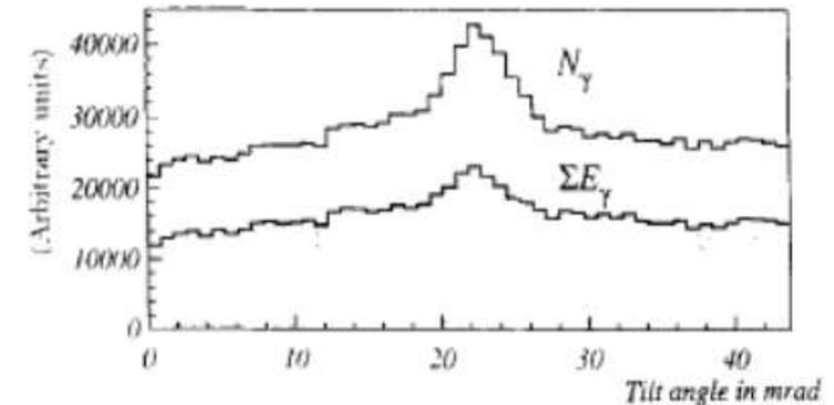
Fig. 11. Photon yield and radiated energy from a 1 mm thick tungsten crystal versus tilt angle between  $\langle 111 \rangle$  axis and electron beam for an incident energy of 2 GeV. Rotation axis is the vertical one, the collimation angle is 1 mrad (from Ref. [14]). Both curves are represented in arbitrary units for the vertical scale.
