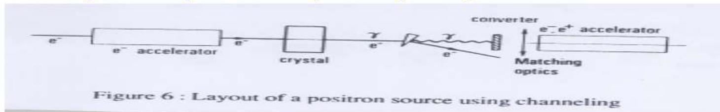
Simulations of an hybrid source made of Ge or Si crystals as radiators and amorphous W as converters:
