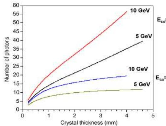
Fig. 2. Total photon yield versus crystal thickness for incident energies of 5 GeV and 10 GeV,  $E_{\text{cut off}} = 5$  MeV: upper curve 50 MeV: lower curves.
