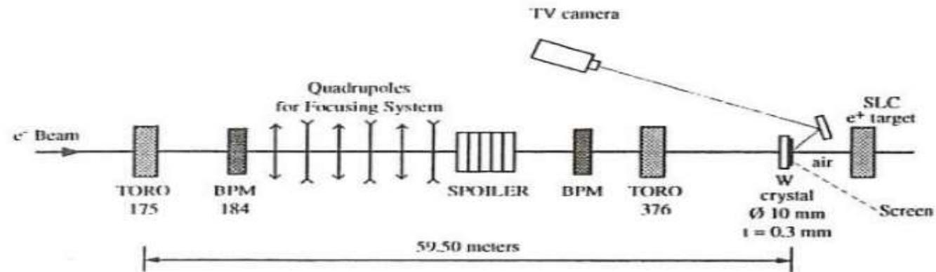
Figure 3: The SLC experimental set-up
