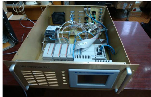
Fig.5.13.23 Chassis with PLCs to control the vacuum of the beam transport line from the linac to the booster.
