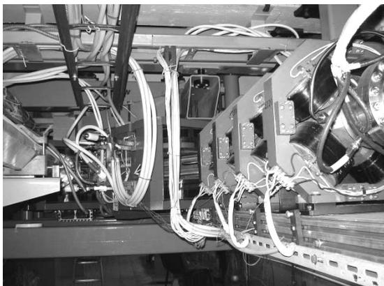
Fig. 6.4.9 Small quadrupole lenses (in the foreground, right) and the small bending magnets (in the background)
