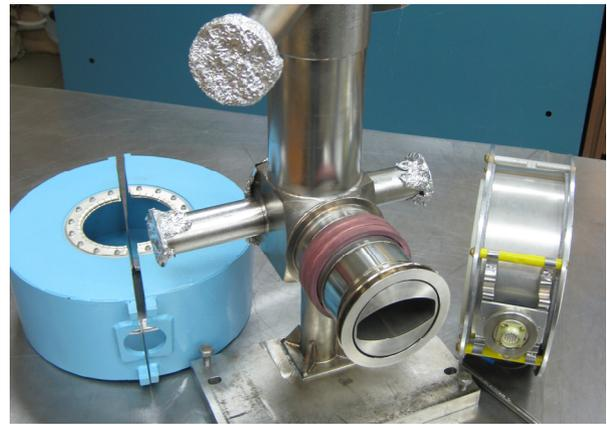
Fig. 5.3.3. Stored beam current sensor of the damping ring before installation on the ring.
