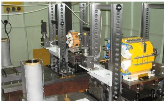
Fig.5.13.6. Two additional benches with rotating coils were constructed for the measurements of the quadrupoles and sextupoles.
