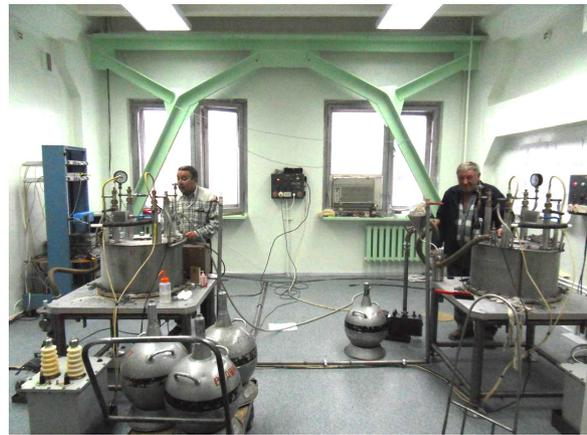
Fig. 4.1.21. Adjustment of the cryogenic magnets for the gyrotron modules.
