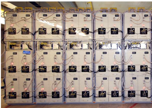
Fig. 5.4.2. View of the pulsed high-voltage power supply for LIA-2.
