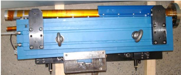
Fig.5.13.16. Extraction "septum magnet" with the vacuum chamber (top view).
