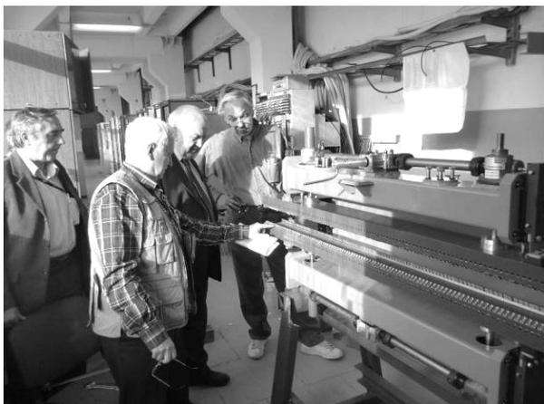
Fig. 6.4.10 Assembling one of the three undulators of the third stage.
