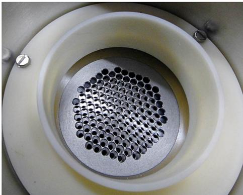
Fig. 4.2.14. Multiaperture diode-type EOS, view from the anode side (beam transport tube is removed).
