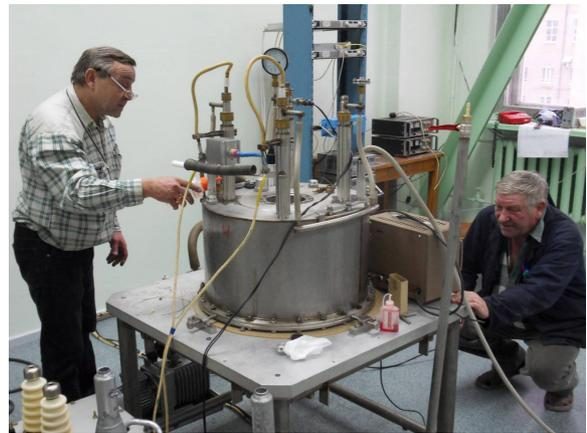
Fig. 4.1.22. Photo of one of the mounted cryogenic magnets, prepared for testing and installation of the gyrotrons.
