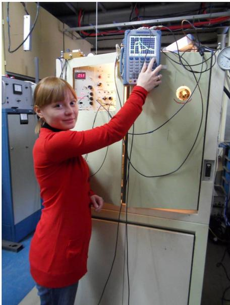
Fig.4.1.24. Testing of the pilot version of the high-voltage modulator.
