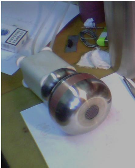
Fig. 4.1.12. Photo of the electron gun, prepared for installation on the GDT: view from the anode.
