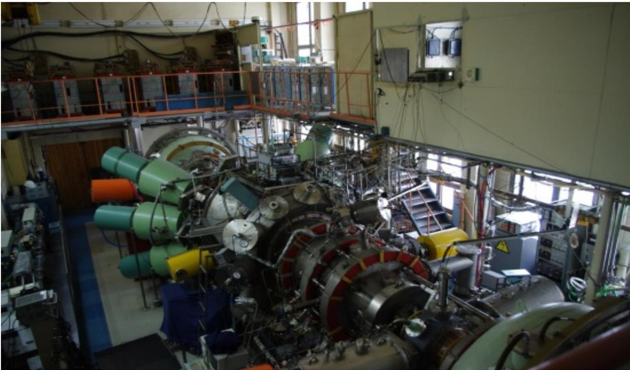
Fig. 4.1.2. View of the GDT facility with two compact magnetic mirrors.
