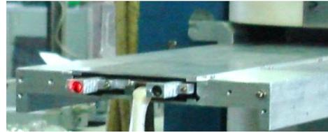
Fig.5.13.7. For magnetic measurements of the dipoles (above), BNL provided a laser tracker and ¼" nonmagnetic corner reflectors, which were mounted on carriages with Hall sensors for the BD and BF dipoles (below). This allowed referring the magnetic measurement maps to the fiducials of the dipoles with accuracy better than 20 microns.
