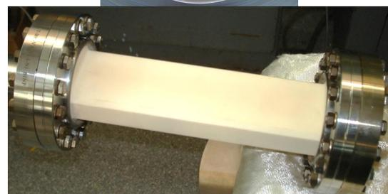
Fig.5.13.19. Ceramic vacuum chamber with the strip coating.
