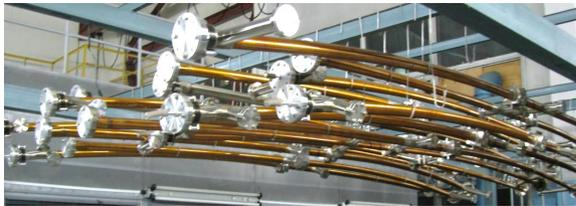
Fig.5.13.9. Completed vacuum chambers. Each is intended for two dipoles and has a pickup.
