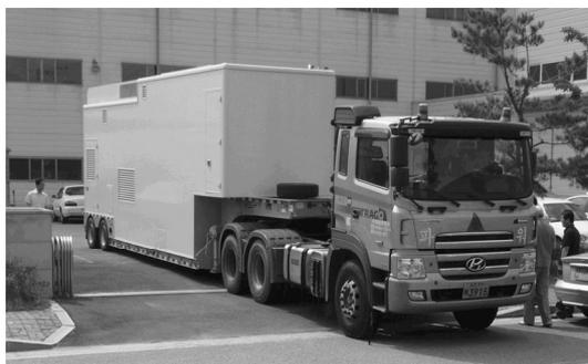
Fig. 8.1.4. Mobile accelerator ELV.
