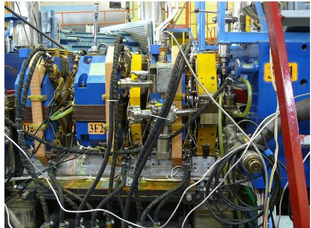
Fig. 5.1.16. Modification of vacuum chamber for Compton backscattering method.
