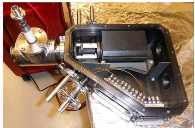
Fig. 4.2.9. Neutral particle analyzer
