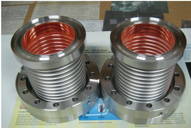
Fig. 5.10.6. Bellows units for the XFEL accelerator structure.
