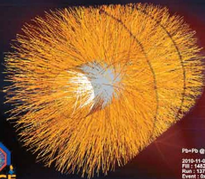
A collision of lead ions provides extensive scientific information: the image obtained by the ALICE detector of the Large Hadron Collider (CERN) shows a large number of traces of the products of the collision of two ions. Such experiments require the maximum possible focusing of ion beams, which cannot be ensured without using the method of electron cooling.
