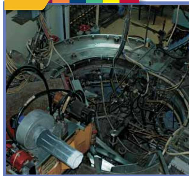
The B-4 booster synchrotron in which there occurs initial acceleration of electron (positron) beams to the injection energy (360 MeV) into the VEPP-3 storage ring
